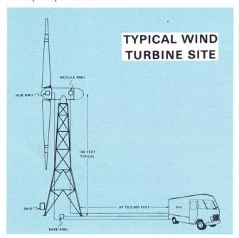
When a Wind Turbine is being installed, a "Maxi-Van" is taken to the site for several months. The equipment in this van allows detailed analysis of data from the new Wind Turbine, and also provides a facility for playback of tapes from other sites.
