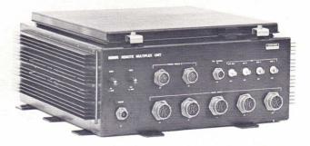
Each signal conditioner output modulates a Voltage-Controlled oscillator(VCO). The 16 VCO's in each group are spaced at intervals of 500 Hz in the spectrum, and zero to full-scale data from a signal conditioner frequency modulates a subcarrier.
