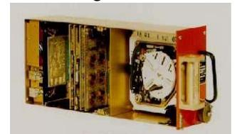
The Fairchild CVR, Models A100 and A100A, manufactured by L-3 Communications Aviation Recorders, were part of this second generation of recorders. They became the most widely used CVR in the world and have now been in service for more than 30 years. During this time, more than 800 aircraft’s have been destroyed in accidents, but the recorders have survived.
