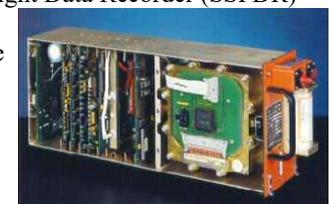
Using the technology of third-generation recorders, operators can extract stored data in a matter of minutes. This data can show how the aircraft has performed in flight, or if a monitored device needs maintenance. Now, the operators of newer generation aircraft can fly with greater safety and reliability. The SSFDR, Model F1000, was the first certified flight recorder to use this new technology.
