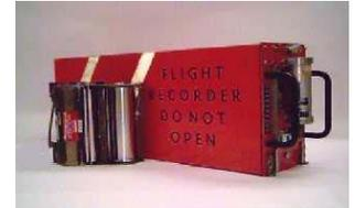
Although most major airlines replaced these old-technology recorders long before required by law, many of these first-generation recorders are still flying in older model aircraft. The remainder of these foil recorders will soon be unusable, since the industry supply of the Incanol steel recording medium has been depleted.
