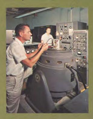
design stages. For example, to assure that all incoming electronic parts meet requirements, parts are routinely aged under cyclic electrical and environmental conditions . . . to provide an added degree of sophistication to EMR's reliability studies, the departments use a general-purpose digital computer to perform simulations of circuit performance as a function of part parameter variations.
