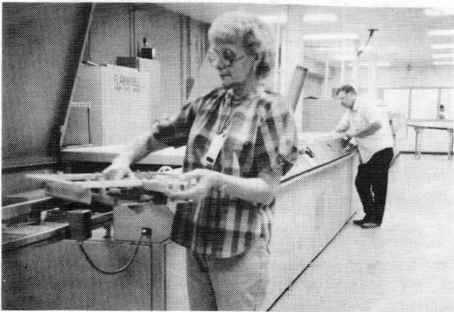
Jean Wilson holds a Printed Wiring Assembly wave solder fixture, preparing to start the Wave Solder System process at the flux unit. In the background, Ronnie Sumner is at the pretrimmer station as Printed Wiring Assemblies are processed through the new Wave Solder System.
