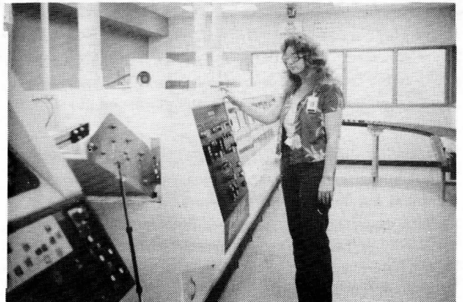
Cheryl Mnick is at the aqueous in-line cleaner portion of the new Wave Solder System. In the background is the conveyor system which returns the Printed Wiring Assemblies to the Wave Solder System's starting point.
