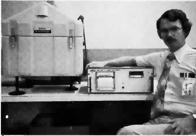
Bob Petrey with Cloud Ceilometer housing (at left) and the ET1504 digital display and strip chart recorder.
