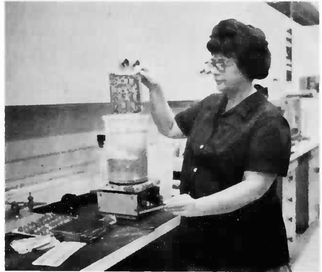
Bonnie Iler, of Materials & Processes Lab, is shown immersing a printed circuit board into gold-stripping solution for salvage.
