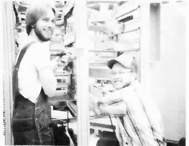
PAT WETJEN (left) and BOB MOORE, Systems Assembly Technician, are shown with some of the complex cables in one of the racks for a flight test system destined for Argentina. "Dressing" cables is one of the tasks performed by our Systems Assembly group.
