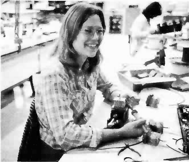
DEBBIE LAHMERS is shown wiring and soldering unibus terminators for CSU (Cyber Service Unit) racks for SWS systems.
