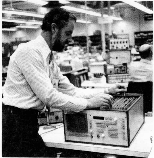
Chris Freeberg, of Test, uses his new "crowbars" to extract tightly-fitting Printed Circuit cards during testing.
