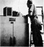
Helen Poirrier at new Scanex Exposure unit in Photo Resist Room, Via this machine, Helen transfers printed circuit pattern to photo resist for development--part of printed circuit board manufacturing process.
