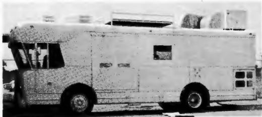
Van-mounted telemetry/computer system will be used in helicopter testing.
