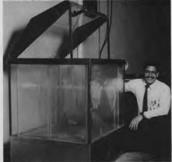
Luis Sandoval with salt fog chamber which simulates the salt atmosphere which shipboard equipments would experience. Actual tests are performed on samples of the materials used in the equipments.
