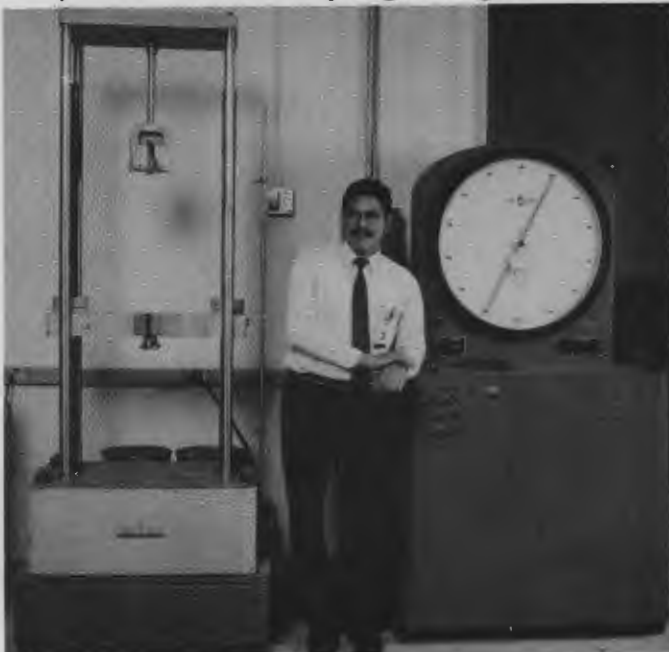
Luis Sandoval with Tensile Stress Tester which pulls materials such as CVR tapes, springs, and also tests weld strength, etc.
