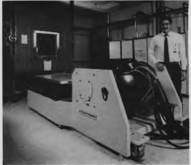
Foreground is "shake" table which performs sine and random vibration testing. Large chamber in background is one of several chambers used for temperature, humidity and vibration tests. Behind Luis Sandoval are amplifiers which drive the shaker. Range of testing: Humidity (20% - 95%); Temperature (-100F to 350F); vibration, up to 100g, depending on load.
