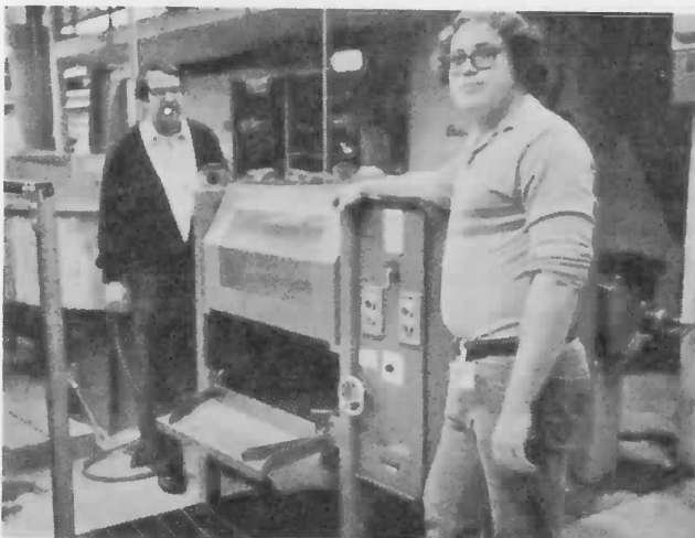
Tom Toler, of Fabrication Engineering, and David Kolchakian, of our Sheet Metal Shop, with new tumbler machine for deburring metal parts.
