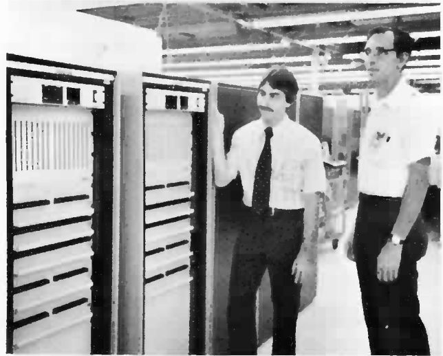
Engineer Mart Dismukes and Technician Milt Litwiller with some RECON III Remote Units -- part of the Los Alamos Supervisory Control system. There are 12 Remote Units in this system.
