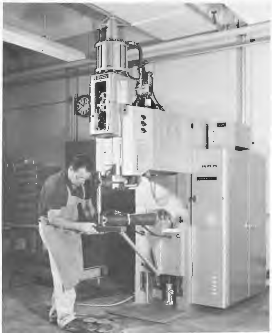
Spot welding on certified three-phase welding machine.
