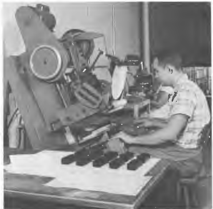
A special printing machine is used to imprint markings on EMR panels and instrument cases.
