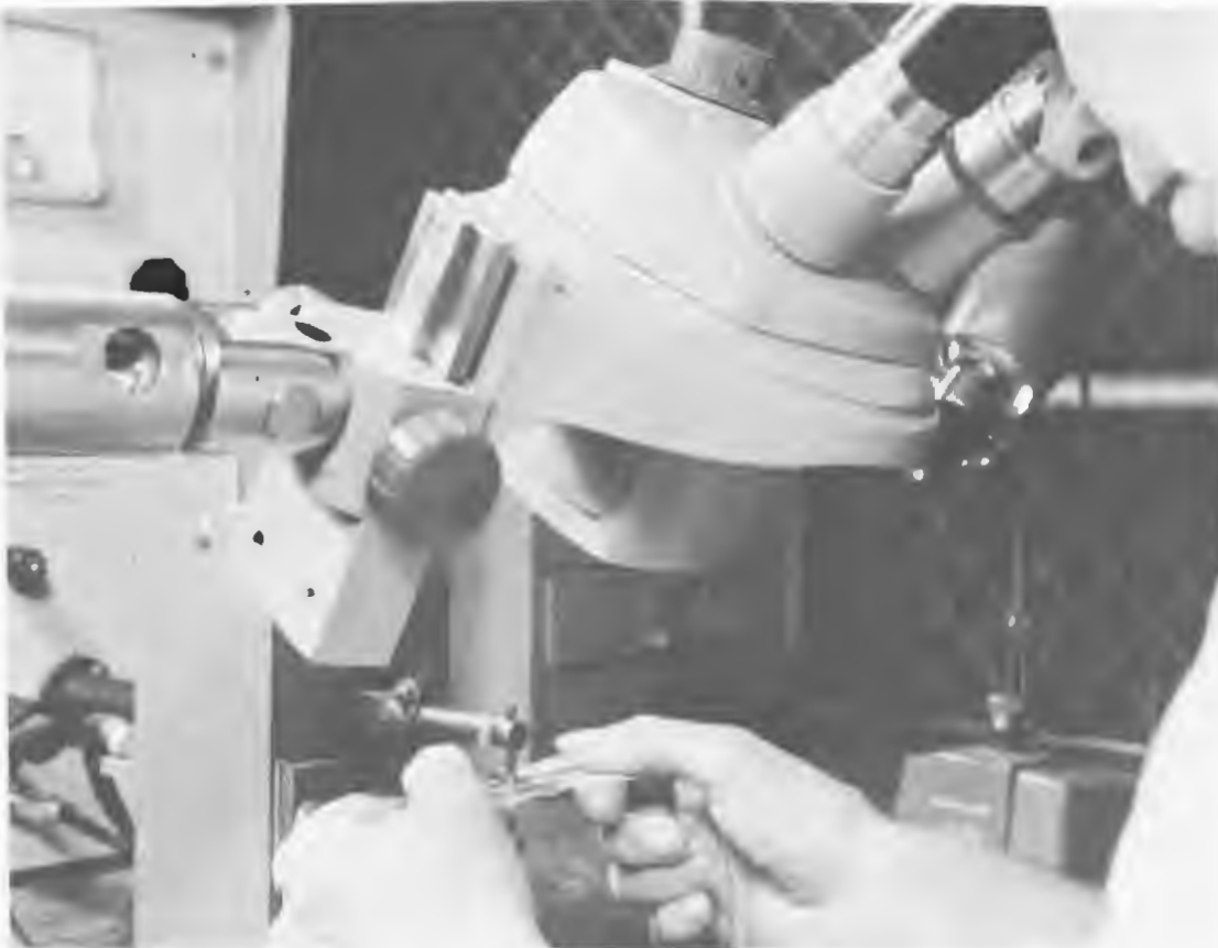
A welded wire matrix is being assembled for a satellite encoder under a binocular microscope.
