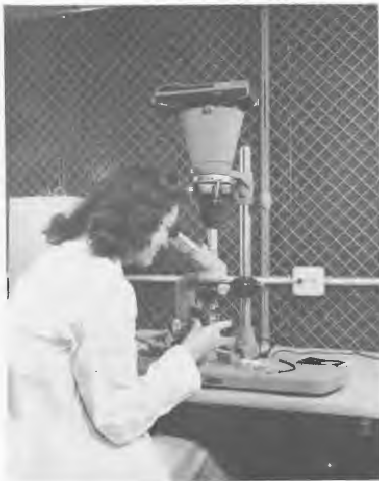
Production welding is controlled by metallurgical analysis. Here a weld is being analyzed and photographed.
