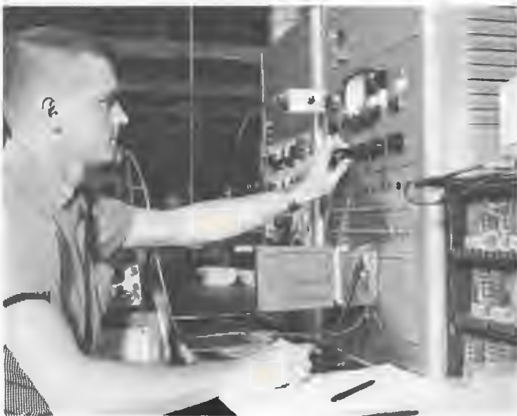
Many special test instruments are built by EMR for checking subassemblies. This test technician is checking a digital decommutation circuit card.
