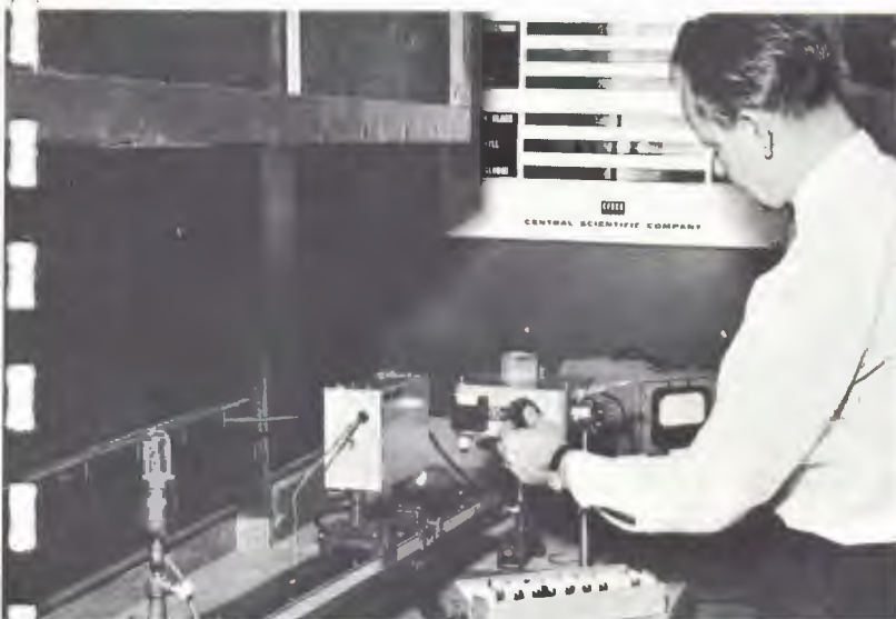
A monochromator is being used to plot the spectral response characteristics of an ultraviolet filter.
