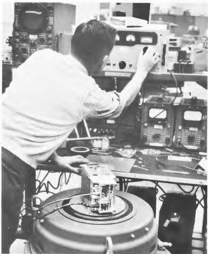
Telemetry transmitter for Mercury under vibration test.
