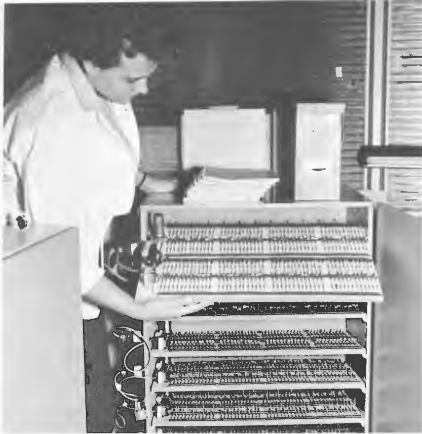
Racks of transistors are electrically cycled to pre-age them before use in critical circuits.
