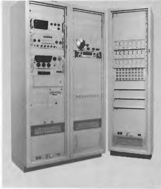
The EMR telemetry systems in the TEL 4 blockhouse at Cape Kennedy include this two-rack discriminator test analyzer and 18-channel discriminator system
