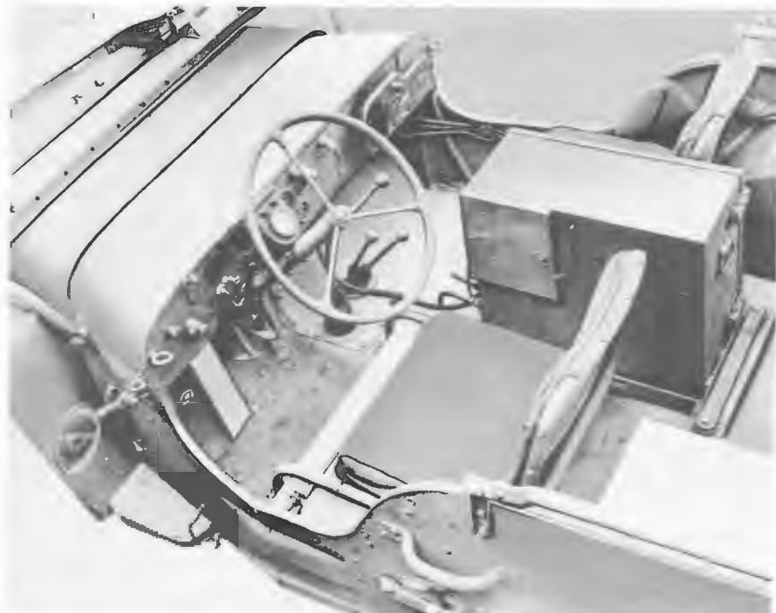
Jeep mounted mine detector developed by EMR automatically stopped jeep.
