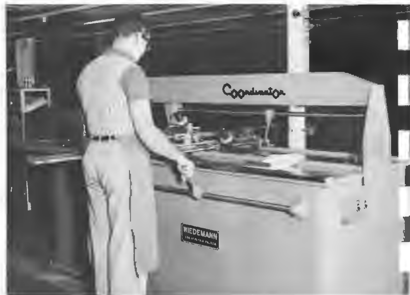
Preparing a precision template on a Wiedemann coordinator.
