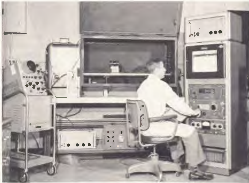
The effect of temperature on the energy resolution of a photomultiplier is being studied with this electro-optical equipment.
