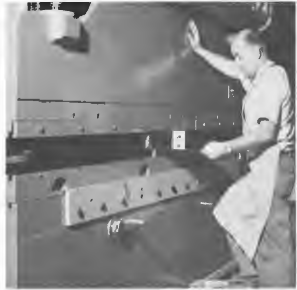
A 60-ton, ten-foot press brake for heavy duty bending and forming.
