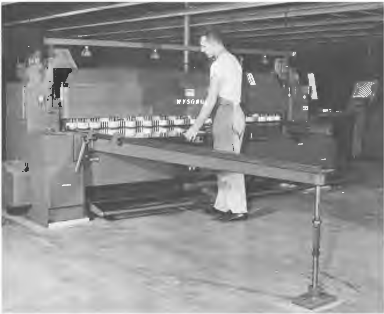
Shearing stock to size in a ten-foot heavy-duty precision shear.
