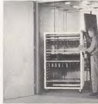
Spray-painted instrument parts are dried in a 6' x 6' x 8' sealed drying oven.
