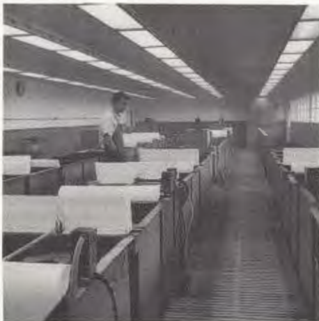
A view of the three EMR plating lines equipped to handle virtually any type of plating on a production basis.
