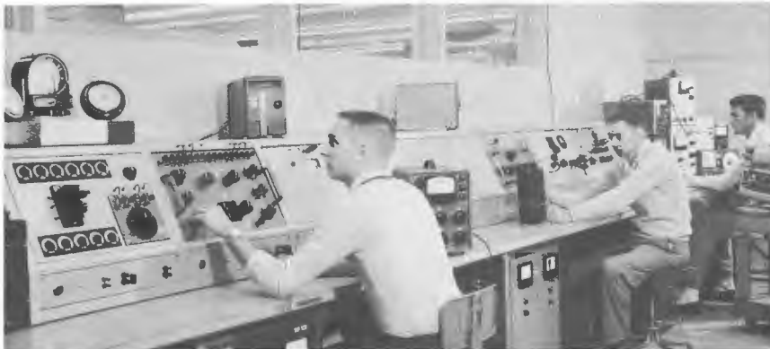
The temperature and humidity controlled Standards Laboratory has a full complement of certified mechanical and electrical primary standards for periodically calibrating all measuring equipment used in EMR product acceptance tests.
