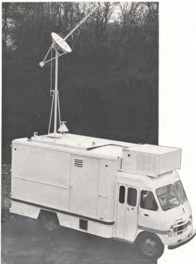
Small telemetry truck constructed for on-the-range testing at the Pacific Missile Range. A tracking antenna is mounted in operating position and the omni-directional two-way radio antenna is below it.
