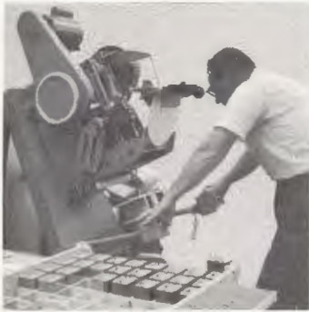
Markem Machine is used to imprint clear panel markings on EMR airborne equipment.
