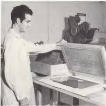
Front-panel silk screen process.
