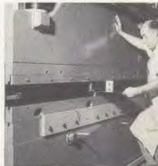
Sixty-ton Niagara ten-foot press brake for heavy duty bending and forming.
