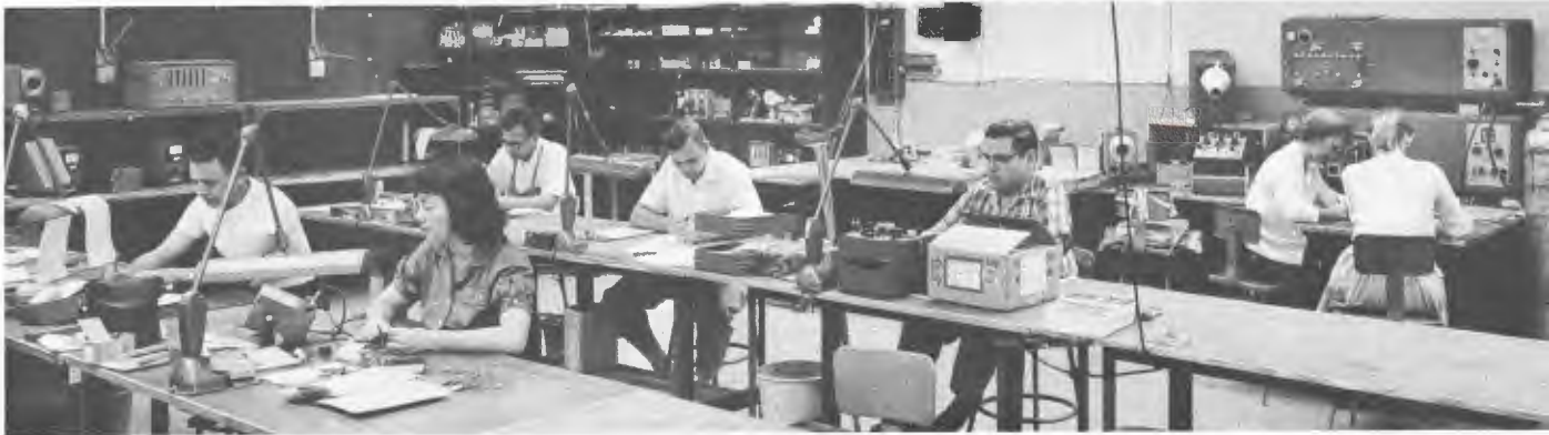
Incoming Inspection area where all purchased material is tested prior to use in EMR products.
