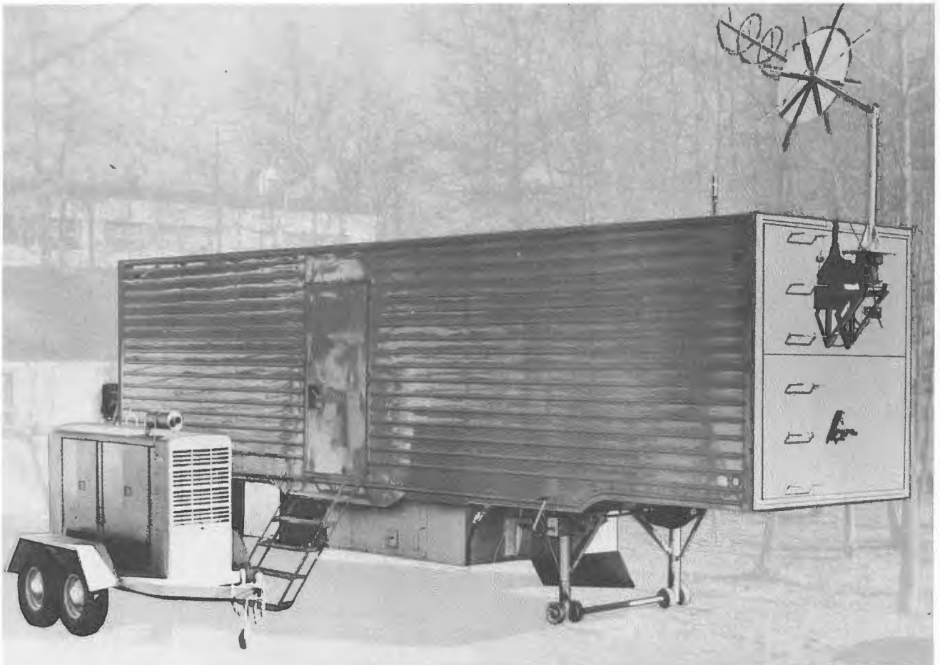
A complete telemetry ground instrumentation station is contained in this large instrumentation van constructed for NAS Patuxent.
