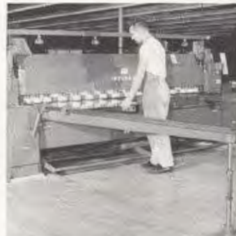
Ten-foot, heavy-duty, Wy-song shear for precision shearing of large sheet metal.
